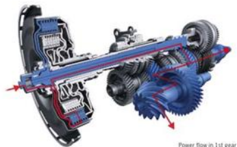
Power flow in 1st gear
