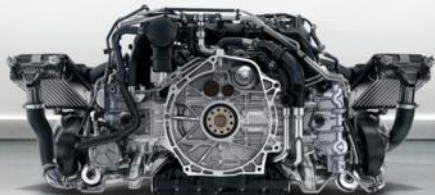
911 Carrera: 272 kW (370 hp), 450 Nm between 1,700 and 5,000 rpm
