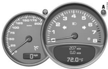
A - Adjustment button for change-over between kilometers/miles
