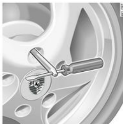
Screw in assembly aid for vehicles without Porsche Ceramic Composite Brake
