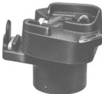
Distributor rotor with speed limiter
