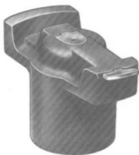
Distributor rotor without speed limiter
