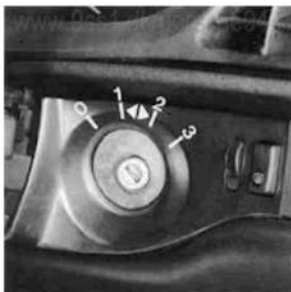
Ignition/Starter Switch with Steering Lock
