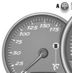
A - Adjustment button for instrument illumination B - Automatic speed control indicator light, Boxster S
