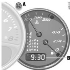
A - Adjustment button for clock B - Clock
