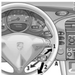
A - Automatic speed control readiness off/on 1 - Set/accelerate 2 - Decelerate/resume 3 - Interrupt
