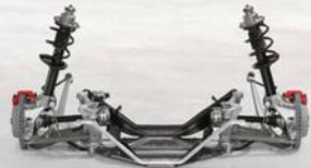
Rear axle with McPherson struts and lateral control arms (Boxster S)
