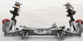
Front axle with McPherson struts and lateral control arms (Boxster S)
