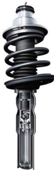
Rebound in 'Sport' mode – working piston only, sporty-comfortable tuning
