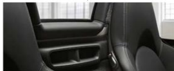
Active subwoofer with 2 x 13 cm low-range speakers and 2 x 6.5 cm mid/high-range speakers
