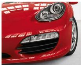
Air intake grilles
