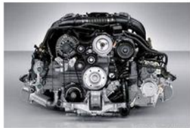
Cayman S: 3.4 litre six-cylinder boxer engine
