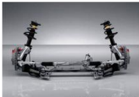
Front side with coil-over strut and lateral control arms Cayman S
