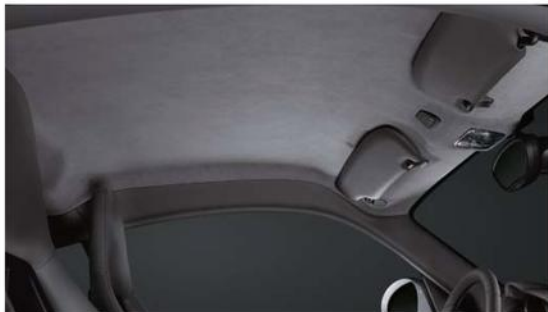
Roof lining in Alcantara
